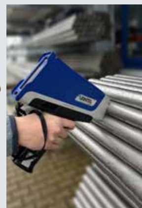
XRF handheld analyzer for the immediate identification of materials and their chemical composition.
