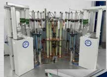
Test laboratory with impulse current generator 200 kA (10/350 \mu s)
